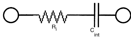
Fig. 1. Simple equivalent circuit for an electrochemical cell with an ionic conductor between two ionically-blocking, but electronically-conducting, electrodes.
